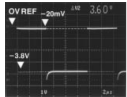
Figure 3-15. Bias/Offset adjusted for -2 V. Load current distributed between the negative and positive-going swings. Peak to peak amplitude remains the same (10% down).
